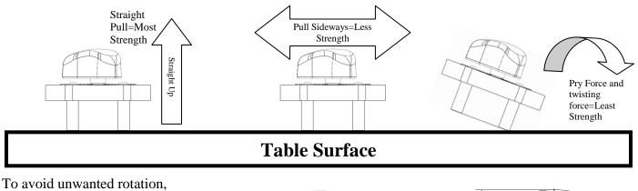
use in pairs at ends of material.
